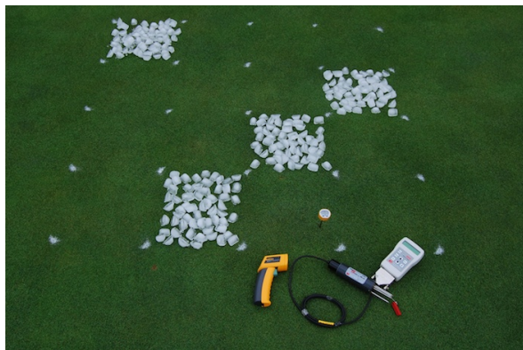
Figure 5: In an experiment conducted on a bentgrass green in Chiba, ice, ice water, and 26°C tap water were applied and the soil and surface temperature were measured.
