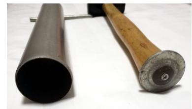
Figure 1: After using many different sampling tools, my favorite is 4 cm diameter stainless steel pipe, slightly sharpened at one end. This type of sampler pulls a clean and compressed core that is easy to cut at exact depth. Samplers with a tapered tip seem to decompact the soil. I have used them for OM246 sampling but prefer straight samplers with no taper at the tip.
