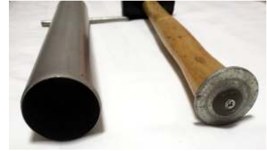
Figure 1: This is a 4 cm diameter sampler made from stainless steel pipe.
