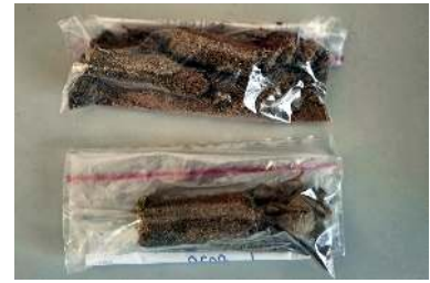
Figure 4: A composite sample (top) and a single core sample (bottom) in adjacent sealed bags prior to shipping.
